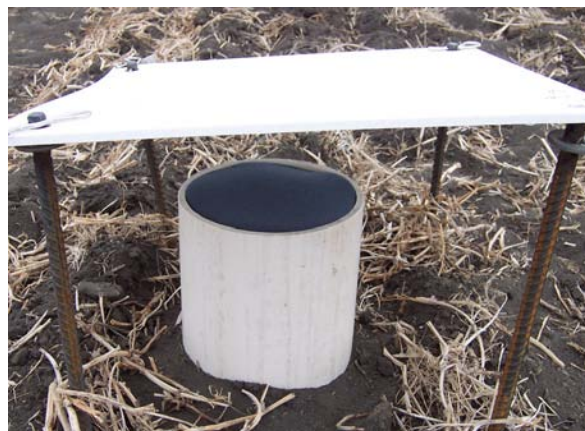
Fig. 1. Chambers used to measure NH 3 emissions from surface applied N fertilizer.
